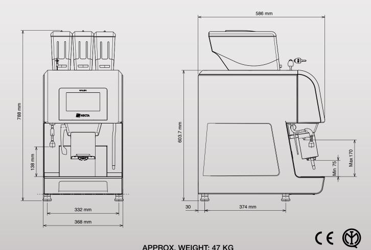
APPROX. WEIGHT: 47 KG ELECTRICAL CONFIGURATION: 230 / 240 V - 50 HZ POWER: 3000 W
